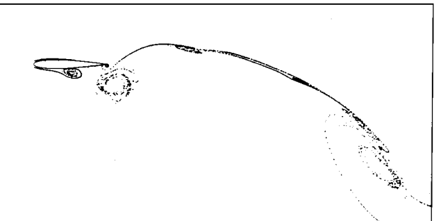
Fig. 4d Unsteady particle traces over a NACA 0012 airfoil oscillated in plunge at k = 0.8 and h_0 = 0.70 .
